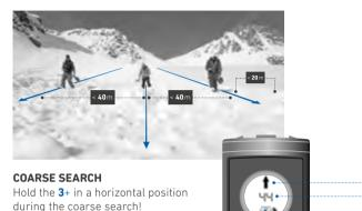
From a distance of approx. 40 m to the avalanche victim, move the direction pointer (4) and distance indicator (5) along the field line to the target point.
