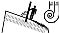
Search for the victim by probing in concentric spirals progressively away from the minimum distance point detected by your ARVA. Probe perpendicular to the slope.
