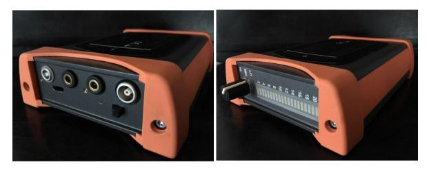
The receiver is housed in a robust Aluminum profile case that is protected by a shock absorber. The front side provides the controls and the display. The rear side provides further controls as well as all connectors.
