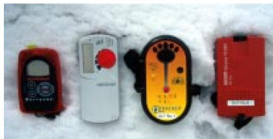
Figure 1: Beacons used in the two tests in February and April 2001 in Switzerland: Mammut Barryvox, Ortovox M2, Tracker DTS and VS 2000 (“old” Barryvox), from left to right, in alphabetical order.
