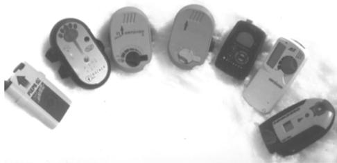
Figure 1: Beacons included in the Austrian test. l.t.r.: Pieps 457, Tracker DTS, Ortovox F1 classic, Ortovox F1 focus, Marmut Barryvox, Ortovox m2, Arva 9000.
