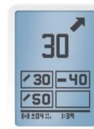
Permanent scan in multiple burials: distance and direction on the basis of 457 kHz
