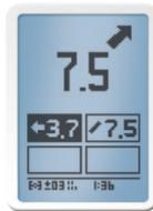
3,7m GPS direction to the marked transceiver
