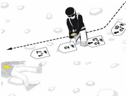
Do an accurate direction adjustment before the direction arrow disappears! You are then moving to the transmitting beacon in best coupling position and save time during the cross-like movements.
