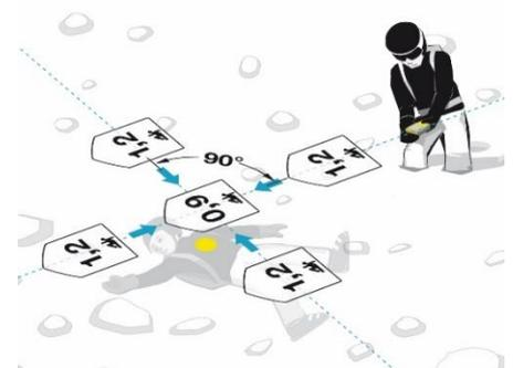
Move your beacon at a slow, steady speed of about 10 cm/s, keep it leveled close to the surface and do not rotate your device. Search along the Y axis, determine the lowest distance value, then follow along the X axis. Always move past the point of the lowest distance to verify the distance tendency. Mark the point of the lowest distance reading and start pinpointing.
