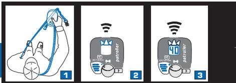
**1 Open the quick lock clasp** and pull the ORTOVOX transceiver *patroller* away from your body for about 1 m. The shoulder strap will still secure the device to your body so there is no risk of losing it.
